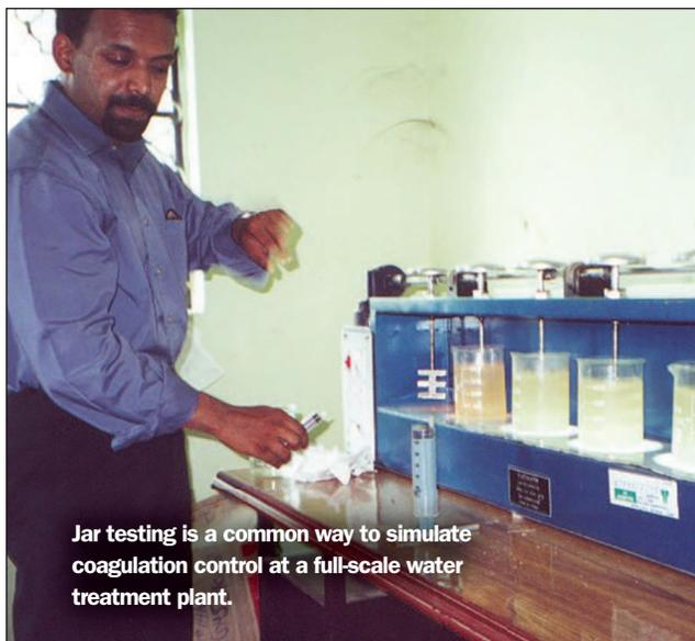
Jar testing is a common way to simulate coagulation control at a full-scale water treatment plant.
